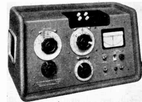
Marconi Instruments H.F. Circuit Magnification Meter using a square-face instrument for its built-in valve voltmeter.
