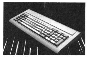
keyboard assembly uses a full-travel membrane keyswitch action with a choice of linear or tactile switching action. Reliability is very high, with typical life cycles in excess of 50 million operations, and the membrane technique provides environmental protection for the switching elements.
