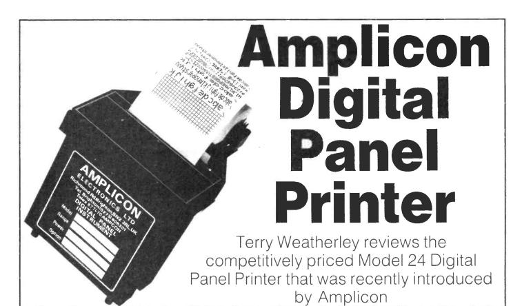
This printer is a neat unit that is intended to be built into equipment and will fit either the DIN96 x 48mm or NEMA panel cutouts.
