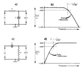
**Fig 18** Circuits and response curves of simple first-order R–C filters. **Parts a,b** refer to low-pass filters; **parts c,d** to high-pass filters
