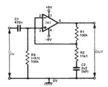
Fig 5 Non-inverting x10 AC amplifier with 100k input impedance
