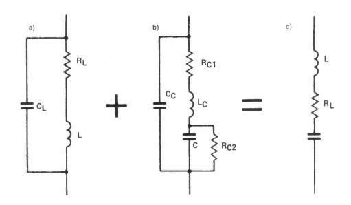
Fig 1: a) Equivalent circuit of an inductor; b)Equivalent circuit of a capacitor; and c) Simplified series tuned circuit
