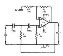
**Fig 23** 'Equal components' version of a 2ndorder 100Hz high-pass filter:  $f_c = 1/2\pi RC$
