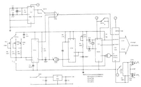
Circuit diagram for LCD capacitance meter
