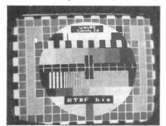
**Photo 1** Belgian PM5544 test card from the Wavre transmitter on channel E28
