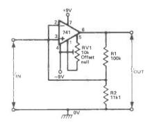
**Fig 3** Non-inverting DC amplifier with offset nulling facility and x10 gain.  $A = (R_1 + R_2)/R_2$ .  $R_{source} = R1//R2$
