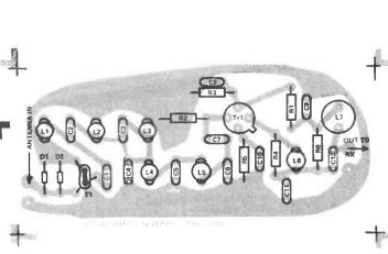
Fig 8 Component overlay
