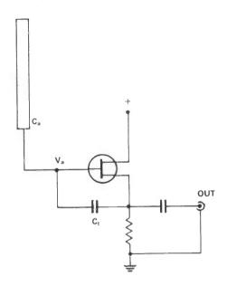
Fig 1 Electrical model of an 'active' antenna
