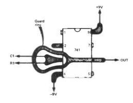
Fig 10 Guard ring etched on a PCB and viewed through the top of the board
