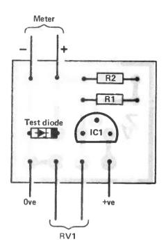
Fig 3: Component overlay
