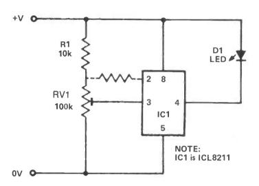
Fig 1 Circuit diagram for a voltage level detector based on a 8211
