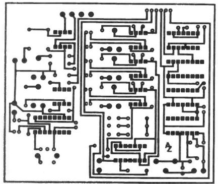
Fig 6: Receiver bottom plane
