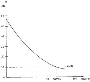
Fig 2 Atmospheric noise related to frequency
