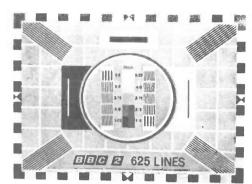
Photo 5 A modified version of Test Card 'C radiated by BBC-2 on UHF
