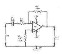
Fig 2 Inverting AC amplifier with x10 gain
