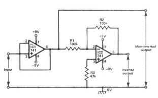
Fig 17 Unity-gain balanced DC phase-splitter
