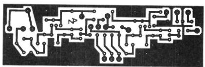
Fig 3: Foil pattern for Q-meter
