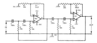
Fig 24 4th-order 100Hz high-pass filter:  $f_c = 1/2\pi RC$
