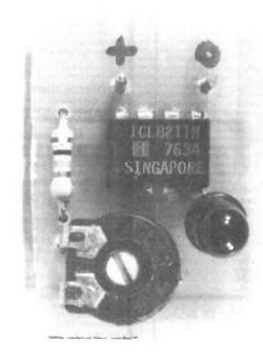
This little project concerns the detection of voltage levels, and how a warning can be given whenever the level rises or falls significantly. Intersil produces two ICs which can be used in this role – the ICL8211 and the ICL7665. We will consider them separately.
