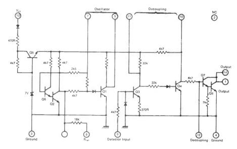
Fig 2: Internal circuit of a ULN2429A
