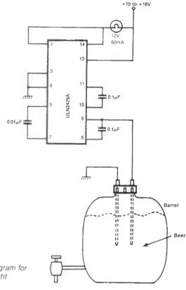
Fig 1: Circuit diagram for the Drinker's Delight
