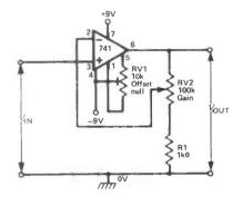
**Fig 4** Non-inverting variable-gain (x1 to x101) DC amplifier
