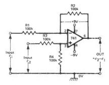
**Fig 16** Unity-gain DC differential amplifier, otherwise known as a subtractor.  $R_1/R_2 = R_3/R_4$ ;  $A = R_2/R_1$
