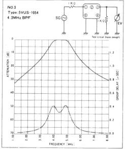
Fig 4: VUS1054 bandpass and test circuit results
