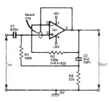
Fig 9 AC voltage follower with 50M input impedance without the guard ring, or 500M with the guard ring
