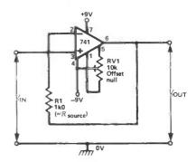
Fig 7 Precision DC voltage follower with offset nulling facility
