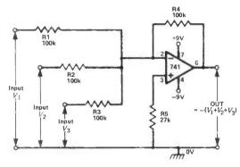
Fig 14 Unity-gain inverting DC adder
