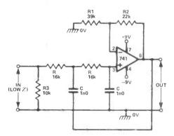
**Fig 20** 'Equal components' version of a 2nd-order 10kHz low-pass active filter.  $f_c = 1/2\pi RC$
