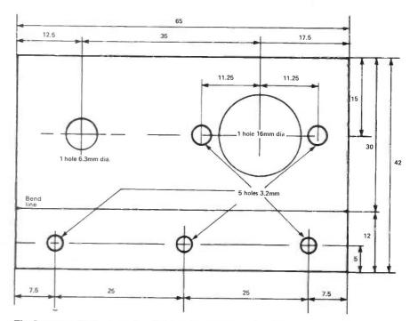
Fig 5: Design for the metal bracket. All dimensions are in millimetres
