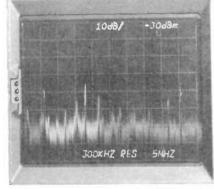
Photo 5: Typical HF spectrum on a wire antenna
