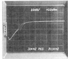
Photo 4: LF roll-off and 455kHz trap effect
