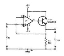
Fig 12 Unilateral DC voltage follower with boosted output-current drive
