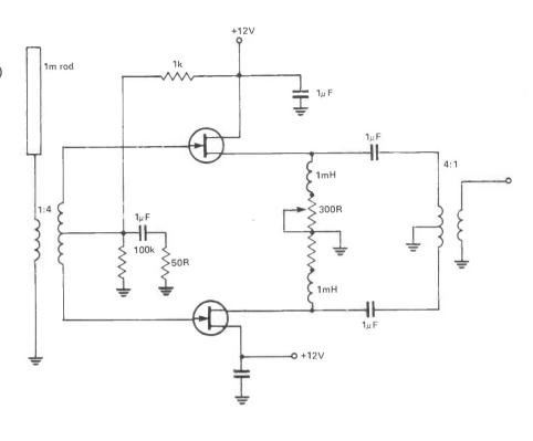
Fig 9 The strong signal active antenna suggested by Ulrich Rhode. The FETs quoted are CP640's, but J310's should substitute adequately for amateur purposes
