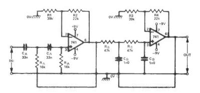
Fig 25 300Hz-3.4kHz speech filter with 2nd-order response
