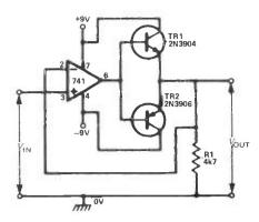
Fig 13 Bidirectional DC voltage follower with boosted output-current drive
