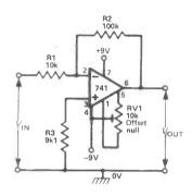
**Fig 1** Inverting DC amplifier with a x10 voltage gain and incorporating an offset-nulling facility.  $A = R_2/R_1$ :  $V_{OUT} = -A \times V_{IN}$ ;  $Z_{IN} = R1$ ; Bandwidth =  $f_1/A$ ; R3 = R1//R2
