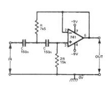
**Fig 22** Unity-gain 2nd-order 100Hz high-pass filter:  $f_c = 1/2.83\pi RC$
