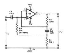
Fig 6 Non-inverting x10 AC amplifier with 50M input impedance
