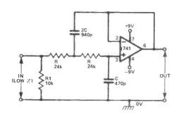
**Fig 19** Unity-gain 2nd-order 10kHz low-pass active filter:  $f_n = 1/2.83\pi RC$
