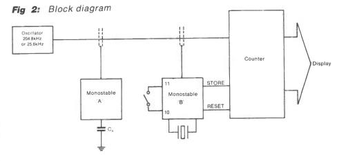
monostable controls gate 'A' in such a way that it turns out that the smaller the capacitor, the fewer pulses get through gate 'A' in the time that gate 'B' is also open. Logic needs to be included to ensure that the two gates are synchronised.
