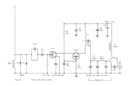
Fig 3: Active antenna head amplifier with low-pass filtering first considered in the November '83 issue
