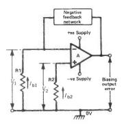
**Fig 11** Input biasing of an op-amp.  $l_{b1} = l_{b2} = l_b$ . Biasing output error= $l_b(R_2 - R_1) \times A = A(V_2 - V_1)$
