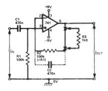
Fig 8 AC voltage follower with 100k input impedance
