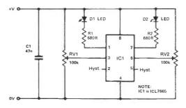
Fig 4: Circuit diagram for detector based on a 7665
