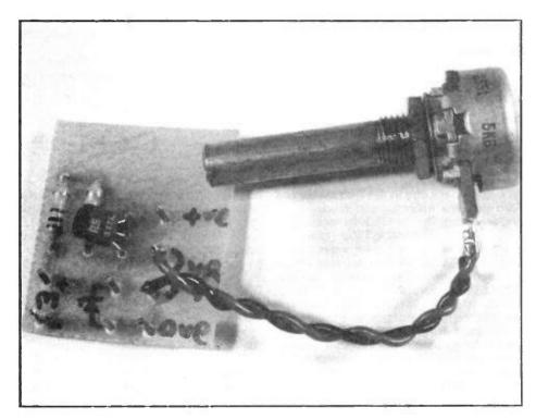
Fig 1: Circuit for the Zener diode checker
