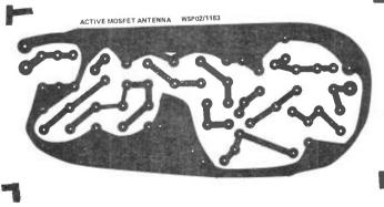
Fig 7 PCB design for the active MOSFET antenna outlined in Figure 4
