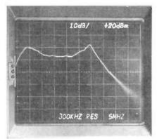
Photo 3: Antenna gain characteristics Centre line = 0dB
