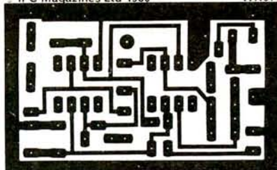
Fig. 11: Modulator printed circuit board (full size)
