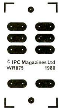
Fig. 15(a): Copper foil layout of the relay board shown full size
