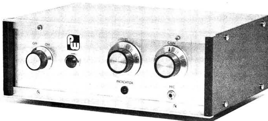
The completed stereo automatic fader unit
