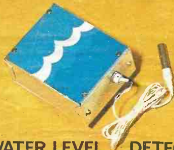
WATER LEVEL DETECTOR
