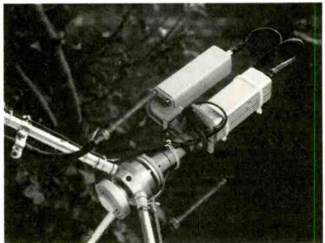
Modifications to the writer's satellite dish include a dual-band Ku/Telecom LNB fitted on the new Chaparrel ortho-mode transducer/polariser.
