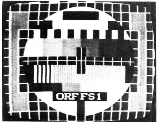
Our heading photograph shows a test card received via single-hop Sporadic E propagation from ORF-Austria by N. E. Parkes, Co. Antrim, using a simple indoor dipole at his home in a block of flats
