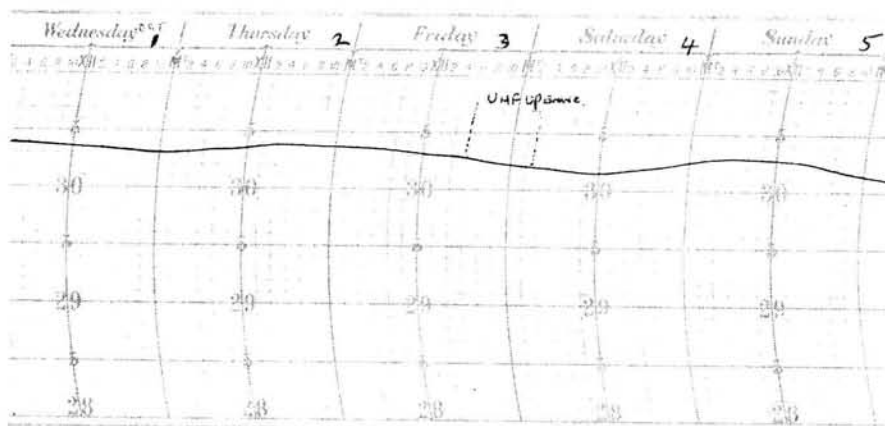
Fig. 4: Barograph chart recorded by the author, showing the change in pressure that caused the extensive tropospheric disturbance on October 3
