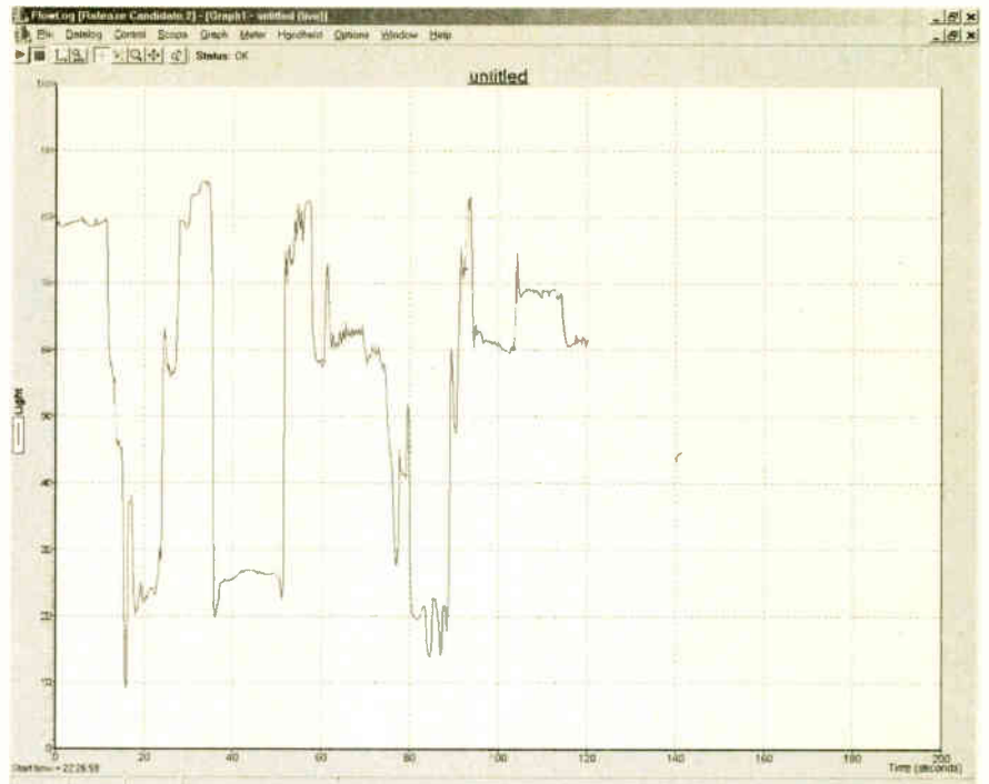
Fig.3. This graph shows the light level received by the built-in light level sensor.
