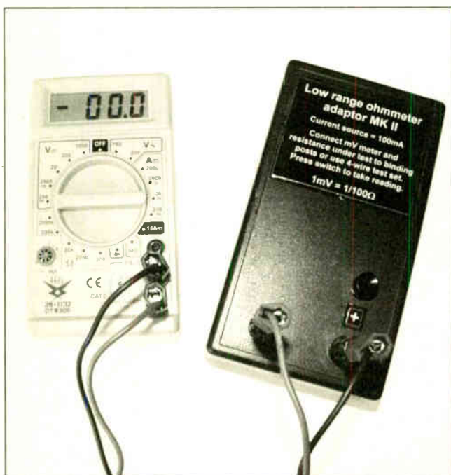
The Low Range Ohmmeter Adaptor Mk2 linked to a Digital Multimeter.
