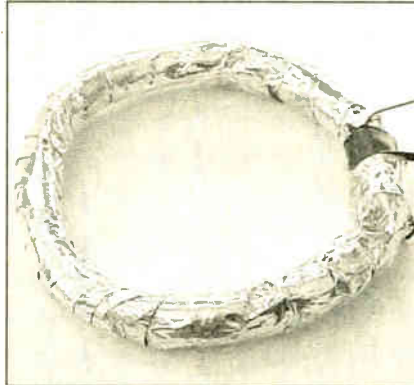
Tin-foil Faraday shield, awaiting final covering of insulating tape.
