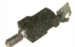
48-141 Good quality vibrating motor as commonly used in the mobile phone and pager industry. Working voltage 3-6V DC. The off centre weight which makes the motor vibrate can easily be removed. Total length 18mm x 6.5mm. Shaft diameter 0.8mm.
