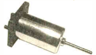
56-141 6V DC motor. Reversible. Approximately 12,000 RPM. Good quality. Square plastic mounting plate with 4 fixing holes on rear of motor. Body size 35 x 19mm diameter. Total length including spindle 62mm. 50p each
