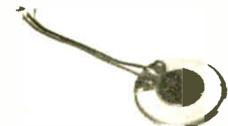
38-433 Mini speaker. Possibly for either headphone or computer use. Measuring 20mm diameter, 3mm thick with a 30mm lead to a 2 pin socket. 28 ohms. 50p each
