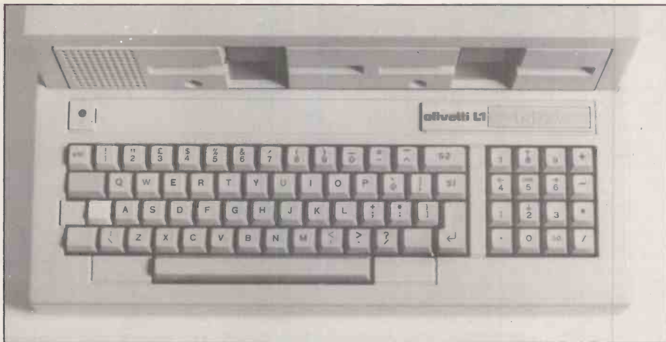
The keyboard is typewriter style with a 16-key numeric keypad added and two curious extra Return keys S1 and S2.
