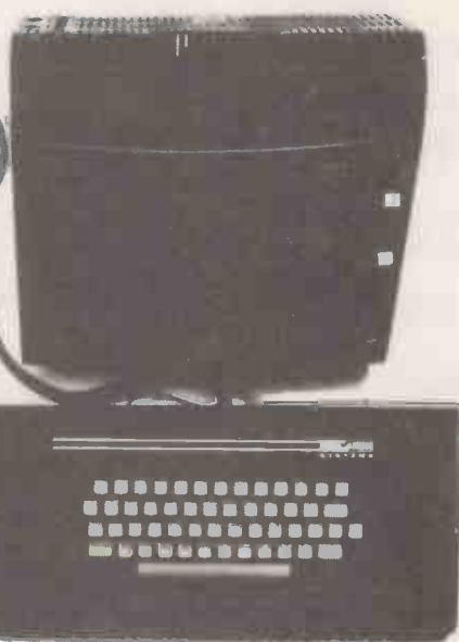
NBZ80-HL. As NBZ80-S, with 16k bytes of RAM, expansion board with 8k BASIC ROM, video interface board, alphanumeric keyboard, book "BASIC Programming Primer". (TV monitor is optional).
