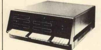
A MINI COMPUTER using MICRO technology at a ridiculous MICRO Price!!! The front panel with a backplane and power supply accepts S100 bus boards from many manufacturers.
