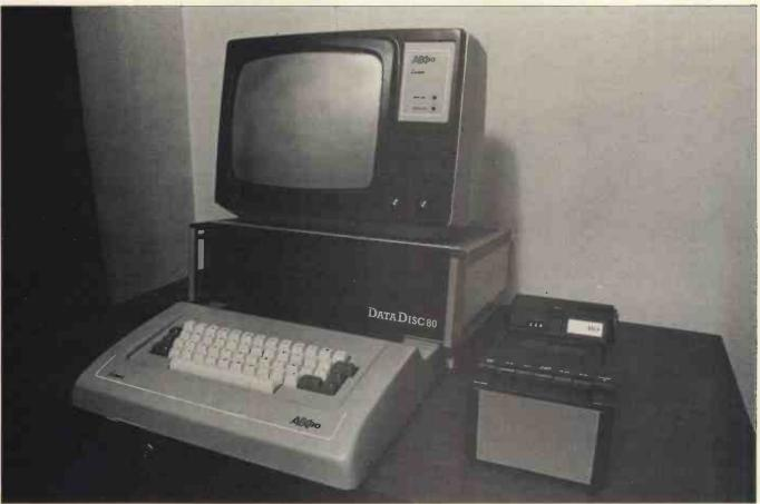
The ABC 80 is based on a single board computer. It contains a Z80A CPU, BASIC in 16K of ROM, 16K user RAM (dynamic), 1K Video RAM, a real time clock, a USART and a PIO. This board is within the keyboard case. On the back of the case there is room to connect a cable to a Databoard 4680 bus, an RS232 port, a reset button, and cables to both the cassette and monitor. The keyboard box is well ventilated and solid.
