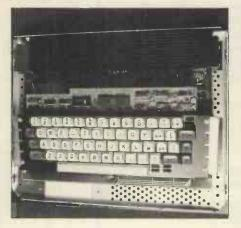
sturdy keyboard, uncluttered by any 'funny' graphics characters is more likely to suit a typist than several of the other lower priced word processing systems. On the back of the keyboard there is a socket suitable for a golfball or daisywheel typewriter.
