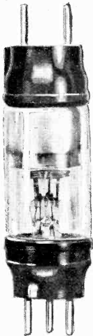
This photo very clearly shows the greater part of the internal construction of the Osram and Marconi S.625. Below is the grid and filament assembly, and above is the screening grid which envelops the anode.
