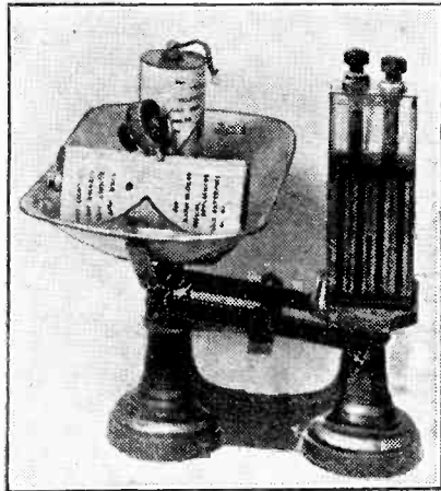
An unspillable accumulator takes less space than dry cells, and weighs only one pound more than the dry. Also there is a filament resistance, which, of course, is not needed when the accumulator is employed.
