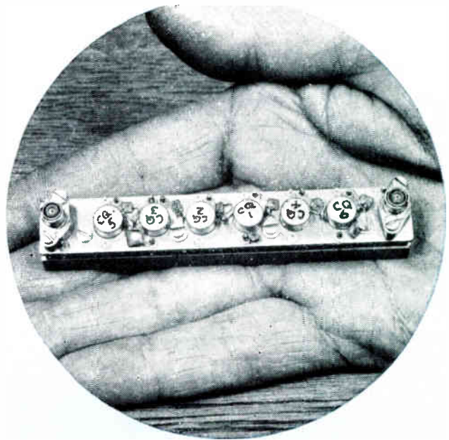
(Right) Five-stage 5-Mc/s amplifier with 60 dB gain and 300 kc/s bandwidth
