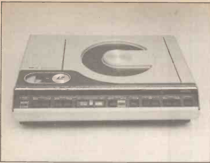
Philips' LaserVision is the favoured technology for interactive video systems, though the Long Play version shown here would not be suitable.
