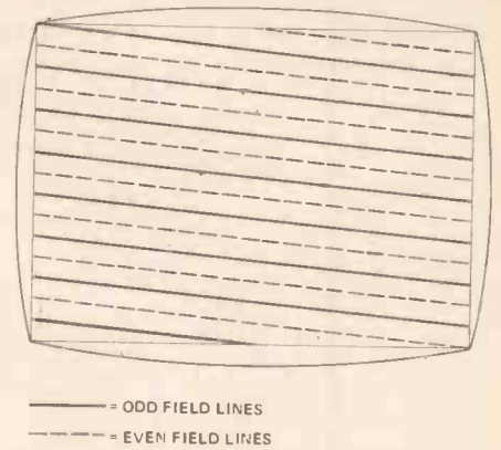
Figure 6. A single raster of lines, used in the UK 625-line television system, composed of two separate fields.
