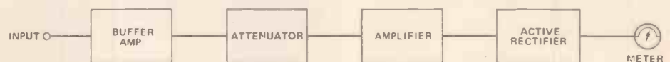
Figure 1. The block diagram of the Audio Millivoltmeter. This circuit is not quite the simplest form of millivoltmeter available: the circuit has been designed to give first-class performance while avoiding some of the problems associated with simpler circuits.
