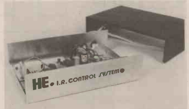
The receiver in its aluminum case. A simple design like this looks unobtrusive.
