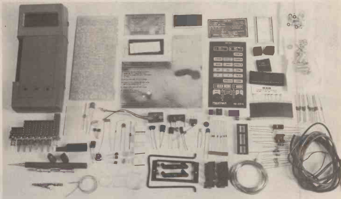
The bits and pieces which make up the Heathkit IM 2215 digital multimeter.
