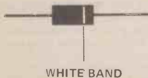
Fig. 1.7 The diode. The cathode end is marked by a white (or black) band.
