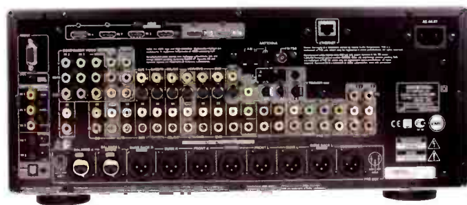
Rear panel looks like a receiver, but has no speaker outputs. Instead it's dominated by eight large XLR outputs and two inputs. There are phono outputs too.
