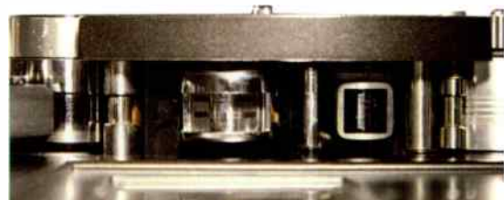
excellent heads mounted on clever detachable head block made the Technics RS1500 series popular with professionals...
