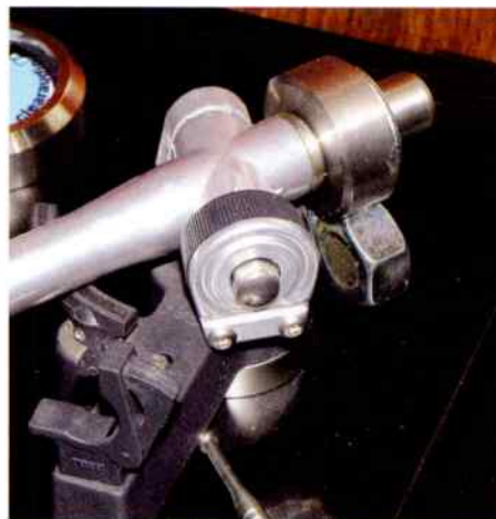
Fix a nut beneath the Rega counterweight and you get better sound, says Denis Holliday.
