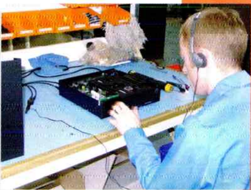
The single-station build concept means one person assembles, tests and packs each product. Diametrically opposed to 'Fordist' mass production techniques, Linn says this approach is essential for quality.
