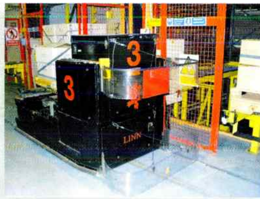
Automated Guide Vehicles distribute materials to work stations around the factory floor. The AGVs follow cables buried under the floor and are controlled by a central computer
