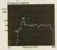
awkward load. Sensitivity was good at 88dB for 2.8V input (nominal watt). They need a moderately powered (around 40W) solid-state amplifier. NK
