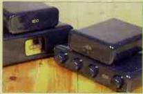
DPA's high-end power amplifiers include the loudspeaker cable in their feedback loop to increase damping factor and improve sound quality.
