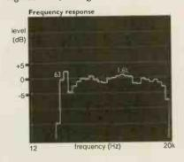
10kHz. These speakers are a light load and need little power, but they are also heavily reactive around 80Hz, which doesn't suit all amps.
