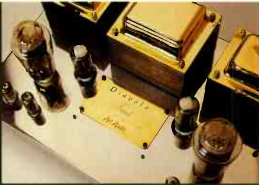
Art Audio single-ended amplifier with Vaic valves
