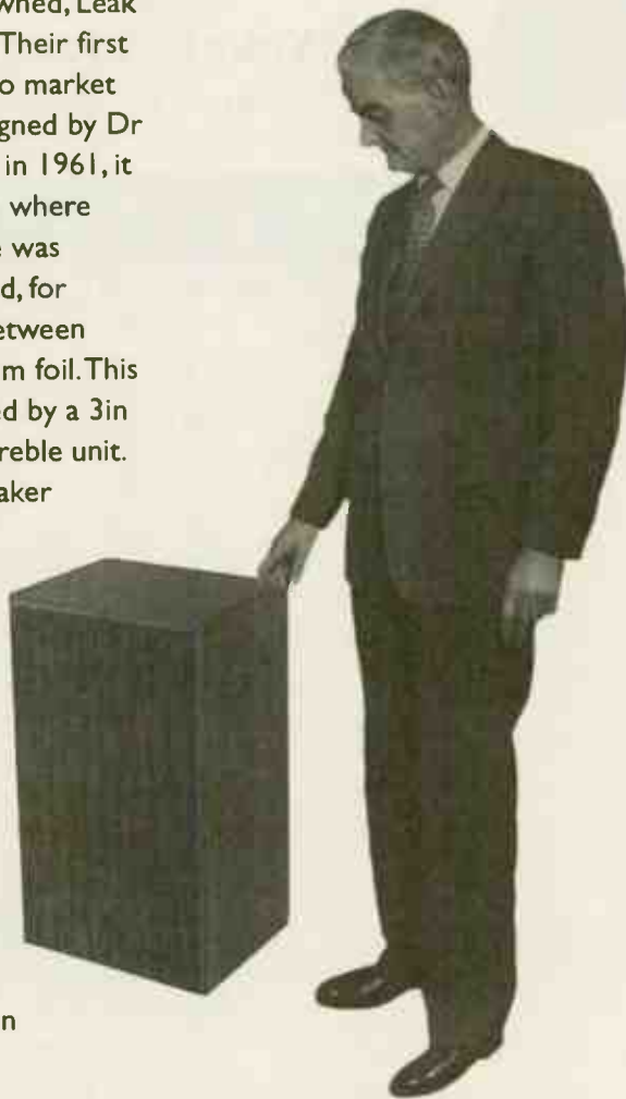
Harold Leak with the company's first 'speaker, the two-way Sandwich introduced in 1961. It used a 13in bass driver and 3in mid/treble unit. The Sandwich 600 followed it.
