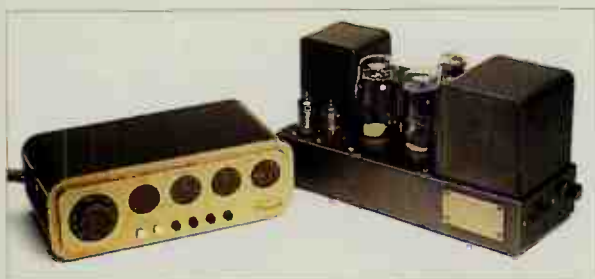
The Quad II produces just 8-10 watts, but it's enough to drive efficient loudspeakers in small rooms - if you don't expect high levels
