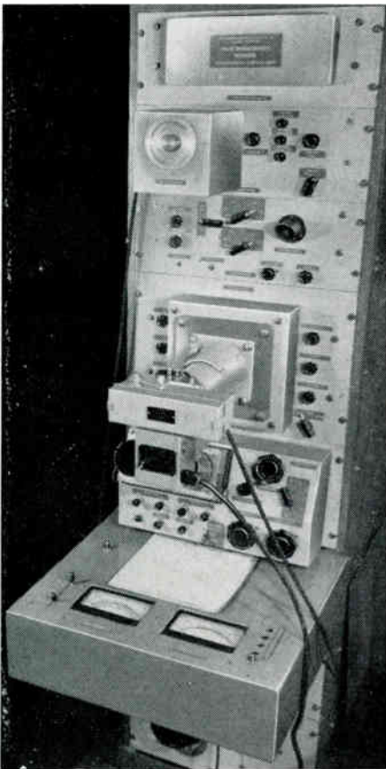
Fig. 7. Experimental display unit of the valve-characteristic recorder.
