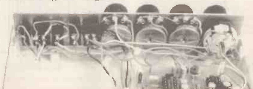
Wiring to front panel controls and output socket.
