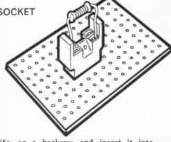
with a sharp knife, or a hacksaw and insert it into your circuit, it becomes a simple matter to remove components and make any necessary substitutions, see diagram.
