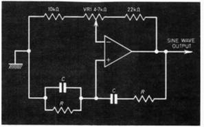
Fig. 1 (left) A simple operational amplifier. The graph shows the amount of gain for different values of resistor X. Fig. 2 (above) A Wien Bridge oscillator.
