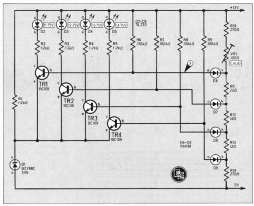
Fig. 1. The complete circuit diagram of the Car L.E.D. Voltmeter. Note that the 12V supply for this circuit is picked up from the car battery supply and that the positive connection must be made to a point after the ignition switch, thus ensuring that there is no drain on the battery with the ignition switched off.
