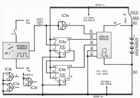
Fig. 8.3. A simple counting circuit to demonstrate the operation of the DISPLAY MODULE, Expt. 8.1.
