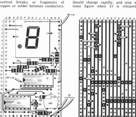
Fig. 2. The unit is assembled on a piece of stripboard. (a) shows the top side with all components in position, (b) shows the underside of the stripboard. Note carefully all the breaks that have to be made in the copper strips. The wiring from the display pins is taken directly to the copper strips. Plastic sleeving should be used for display wiring and all underside links.
