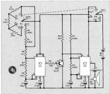
Fig. 2. The complete circuit diagram for the Lightning Chess Buzzer.
