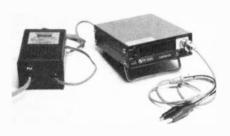
Meter with its input lead and power unit.
