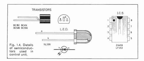
layout; in particular watch the polarity of diodes and the position of pin 1 on the i.c.s. Sockets may be used for the i.c.s as this will be an aid to rapid servicing in the field in the event of failure.
