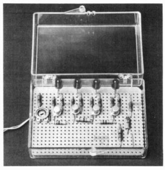
View inside the clear plastic case of the voltmeter showing the push-fit of the stripboard assembly.
