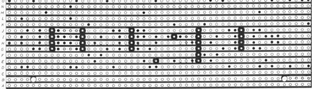
Fig. 2. Stripboard layout of the Two-Tone Horn. Wires marked thus-\* to be omitted if the remote triggering circuit is used. See Fig. 4 for the wiring of this additional feature.
