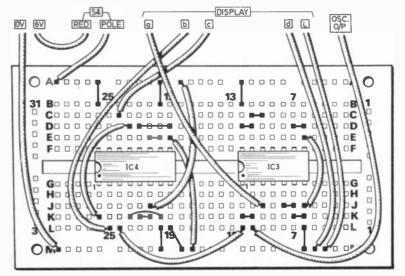
Fig. 8. 4. The layout of the components on the Verobloc for Expt. 8.1.
