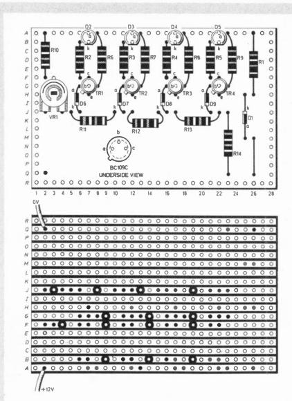
Fig. 2. The stripboard layout for the Voltmeter. L.E.D.s D2 to D5 must be in the positions shown.
