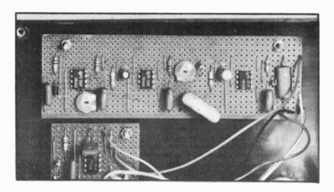
View inside case showing both circuit boards mounted onto the base.
