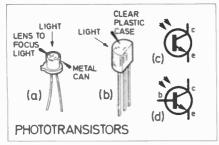
Fig. 8.8. Two common packages for phototransistors and circuit symbols for types with and without a base connection.
