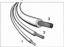
Fig. 1. Examples of equipment wire: (1) 1/0·6; (2) 7/0·2; and (3) 55/0·1
