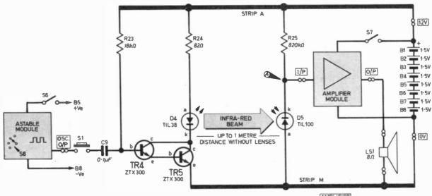
Fig. 8.9. Circuit diagram for a simple infrared communication system. The experiment uses two *Minilab* modules.
