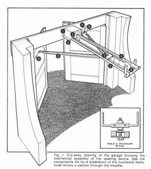
enoid is fitted adjacent to the DOOR FULLY CLOSED microswitch to engage with a large eyebolt with connections made to TB2/3, 4 and 5 on the control unit.
