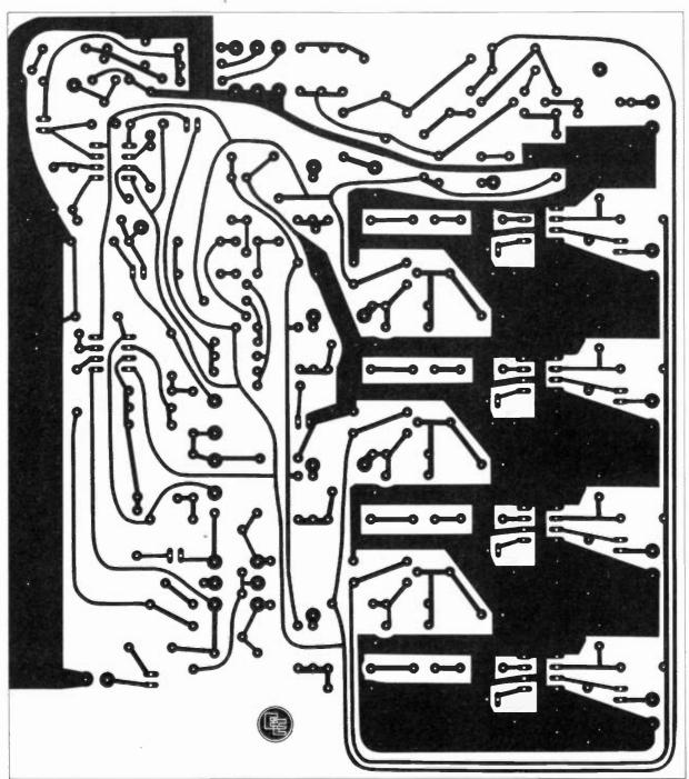
Fig. 1.2. Public Address System: Control Unit printed circuit board, actual size.
