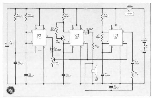
Fig. 1. Circuit diagram of the Two-Tone Horn. Note that S1 and B1 are only required if the remote triggering circuit is not used.
