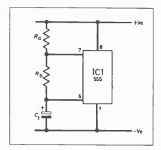
Fig. 1. Selecting the timing values for the Lightning Chess Buzzer.
