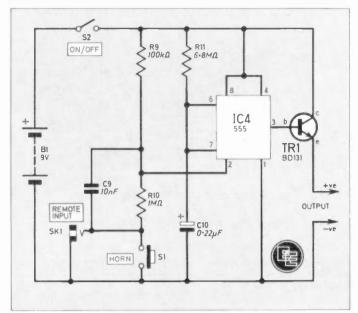
Fig. 3. Circuit diagram of the remote triggering device. The reed switch is connected via  $\ensuremath{\mathsf{SK1}}.$
