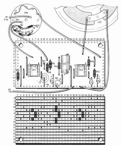
Fig. 3. Circult board component layout and interwiring details.
