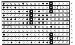
Fig. 4. Stripboard layout of the Automatic Remote Triggering circuit. Refer also to Fig. 2 for the wiring-in of this board to the Horn generating board.
