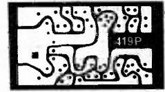
Fig. 4.4. Printed circuit board for the EE Radio Control System Servo Unit, actual size.
