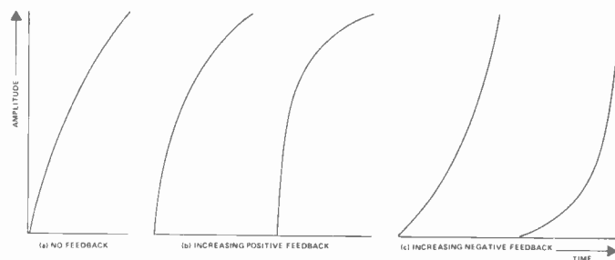
Fig.1. The effect of feedback on the attack response.
