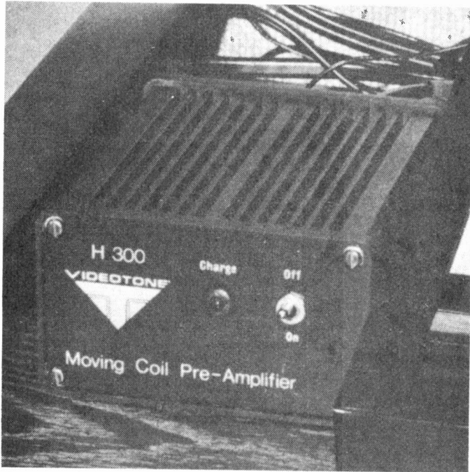
Corals H300 head amplifier which can now be wholeheartedly endorsed because the one fault — a de-thump relay which didn't work on switch-off — has been dealt with by the manufacturer and all is now well.
