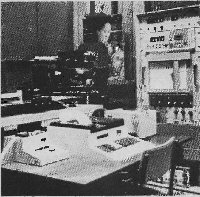
Fig.8. This special spectrophotometer has been developed to monitor changes in colour over long periods.
