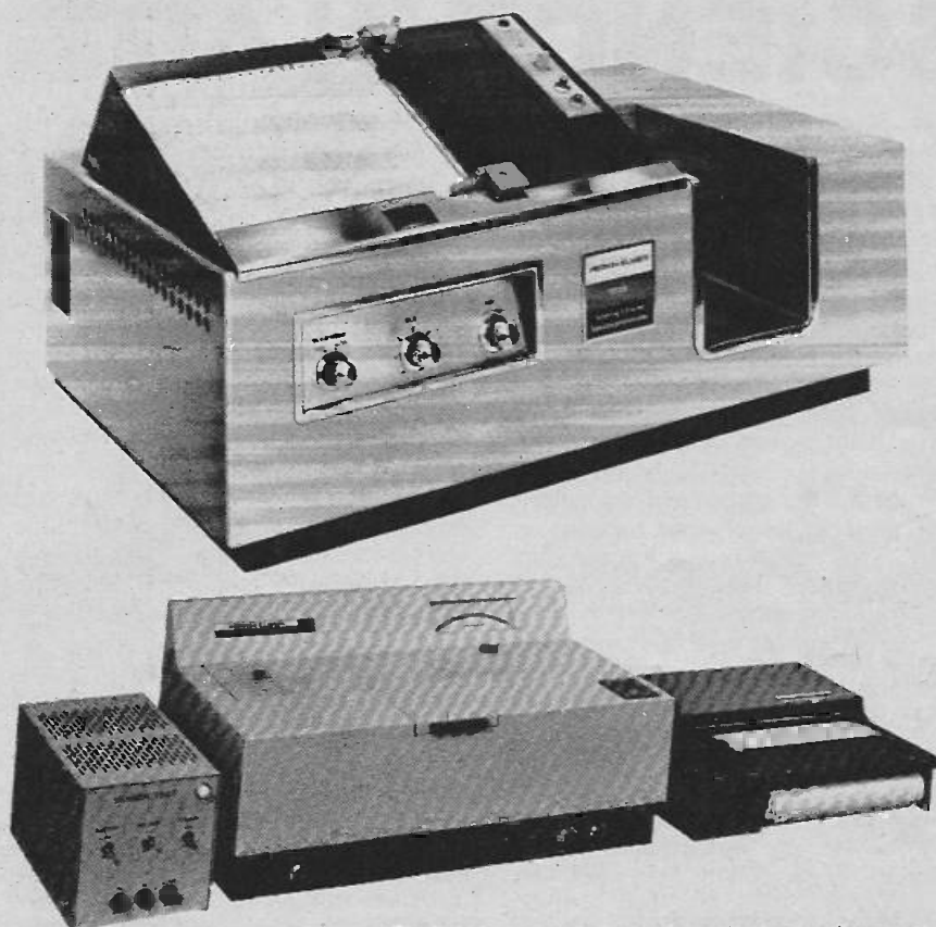
Fig.6. Infrared and ultraviolet radiation studies are made using these Perkin-Elmer spectrophotometers.
