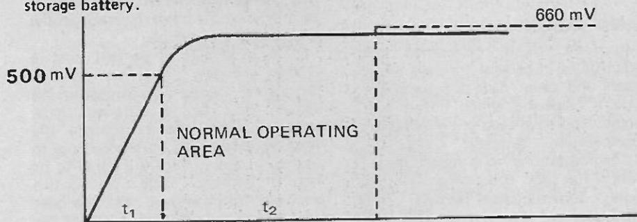
Fig. 1b. Discharge/time curve for ESD at constant current. Normal full charge is to 500 mV. Charging to 600 mV increases operating range by at least ten times.
