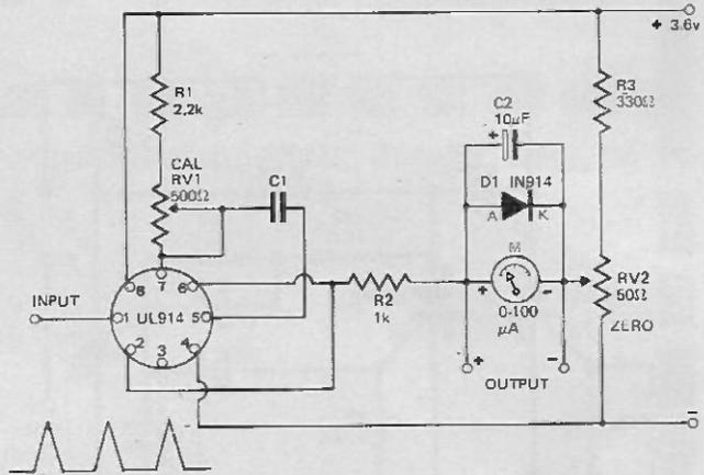
This circuit may be used as a pulse counter, tachometer, or if preceded by a Schmitt trigger, an analogue frequency meter.
