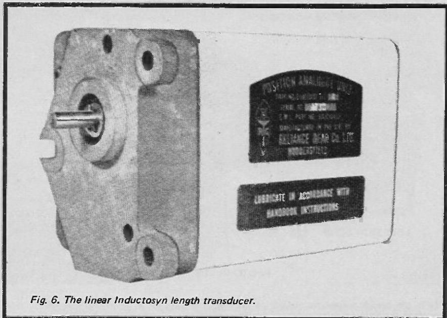
Fig. 6. The linear Inductosyn length transducer.
