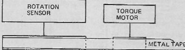
Fig. 4 a/b Alternative tape/wire linear to angular rotation transducers.
