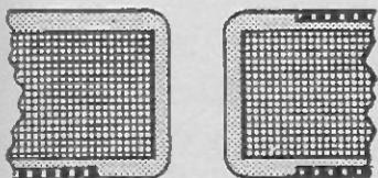
Thick copper plating build-up
