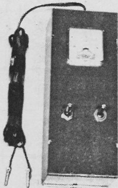
Fig. 6. This device, manufactured in the USA, is specifically designed to detect infinity transmitter devices.
