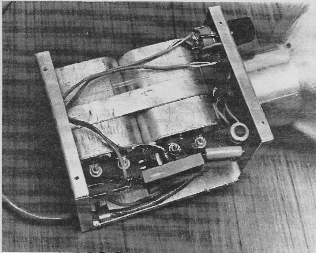
*Fig. 5. Construction of the unit — this particular unit has been constructed to drive two flash-tubes. The additional capacitors and 220 ohm, 10 watt resistor referred to in the text can be clearly seen. The pulse transformer is on the extreme left of the matrix board which in turn is bolted securely to the energy storage capacitors.*
