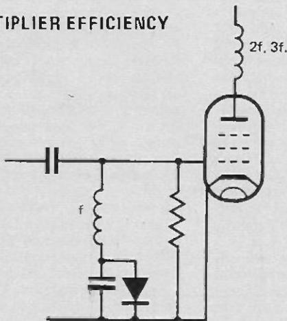
A cheap silicon diode may be used to improve the efficiency of a frequency multiplier.
