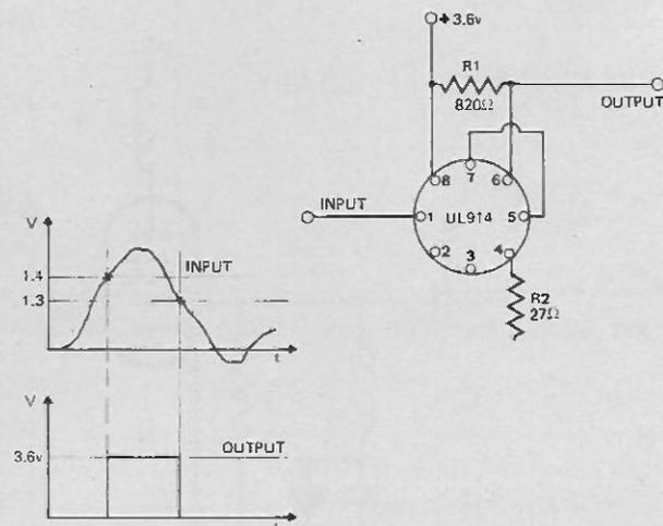
One cheap IC, uL914, can be used as an extremely simple and effective Schmitt trigger suitable for many applications. Hysteresis of the circuit is about 0.1 Volt. This may be varied by altering the values of R1 and R2.
