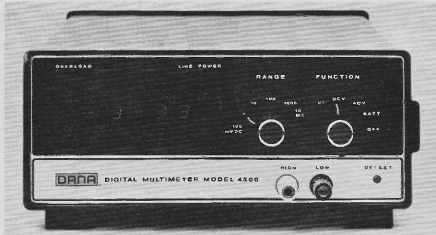
is said to be almost unbreakable physically. It has a case moulded in high-impact plastic, and will withstand far greater shocks and g forces than previous instruments of laboratory standard.
