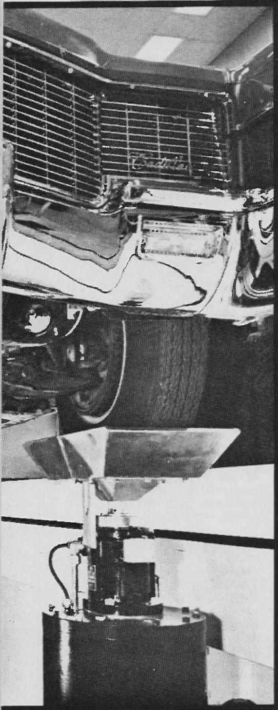
*Detail view of electro-hydraulic actuator, hydraulically operated floor is raised when car is driven onto the simulator, then lowered to allow access to all parts of the car during test.*
