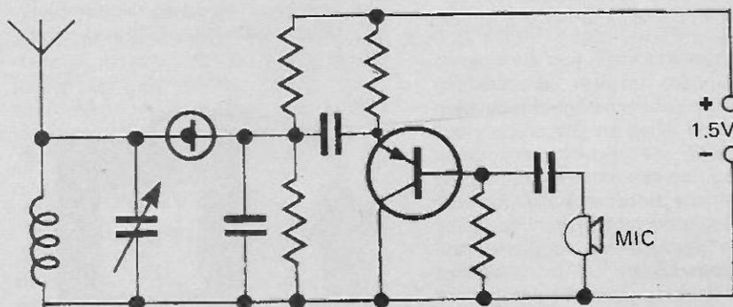
Fig. 7. Typical of simple FM bugs, this device uses a tunnel diode oscillator and radiates in the 90 - 100 MHz band.
