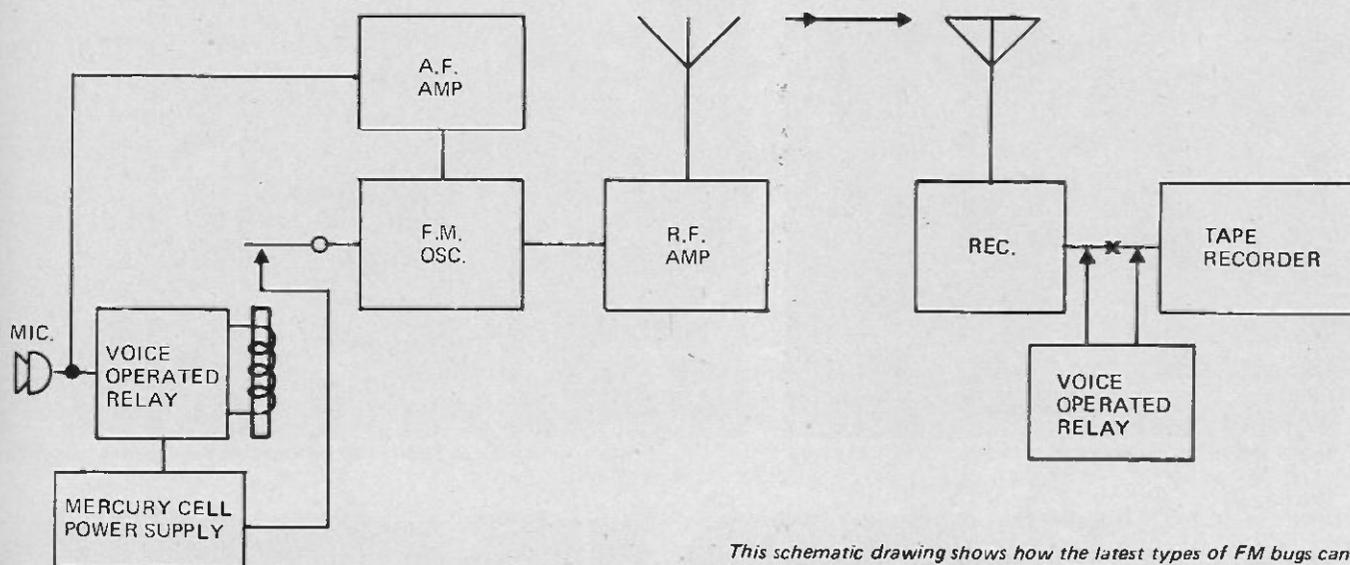
This schematic drawing shows how the latest types of FM bugs can be left unattended for long periods. The voice operated relay on the left of the drawing connects the power supply to the transmitter only during the time that someone is speaking within the room. At the receiving station a second voice operated relay ensures that the tape recorder operates only during signal conditions.
