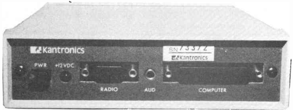
Back view of the TNC, showing the various connections
