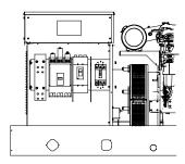
Multiple Circuit Breaker Kit with Neutral Bus Bar 180-300 kW Model Shown
