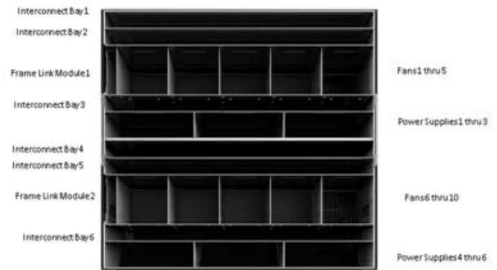
HPE Synergy 12000 Frame - Rear View
