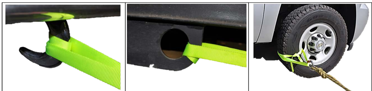
Figure 139- Some examples of vehicle anchor points. L to R. Open hook which requires constant tension to prevent detachment, welded bracket with connection point and attachment directly to a wheel rim (avoiding brake lines) at a right angle.
