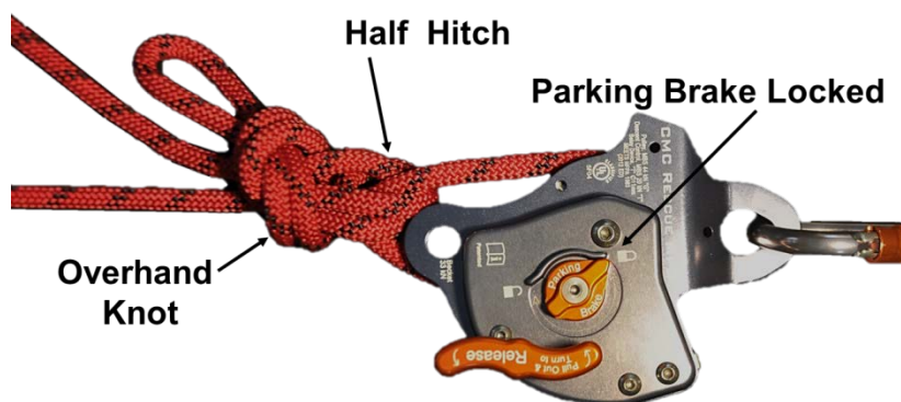
Figure 92- MPD secured with Parking Brake locked and tied off.
