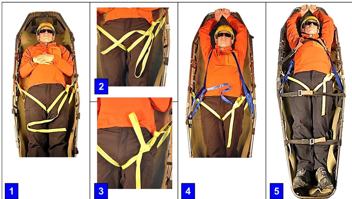
Figure 234- Yosemite litter packaging. Here the pre-existing manufactured cross-tie straps on the litter were incorporated in the patient packaging.
