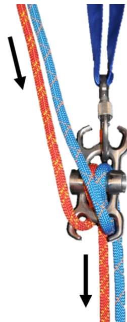
Figure 38- Scarab rigged for a lowering with twin ropes
