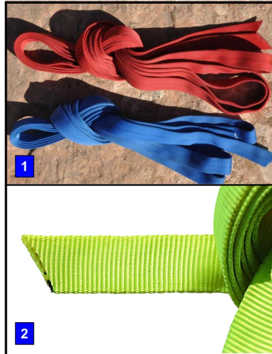
Figure 22- Tubular webbing. 1.) Folded and tied with an overhand knot for storage and easy deployment. 2.) Close-up of webbing with the end cleanly melted to prevent unravelling.
