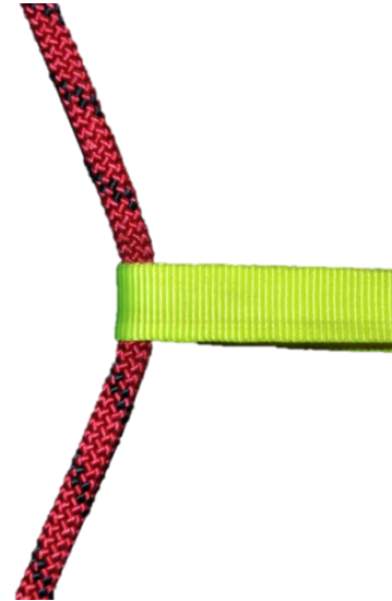
Figure 69- Nylon rigging components rubbing against one another can result in melting leading to failure.
