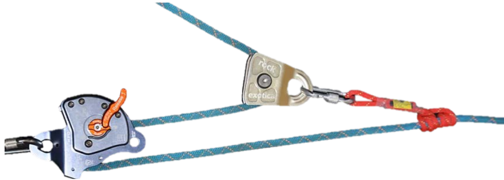
Figure 94- MPD employed in 3:1 simple pulley system.
