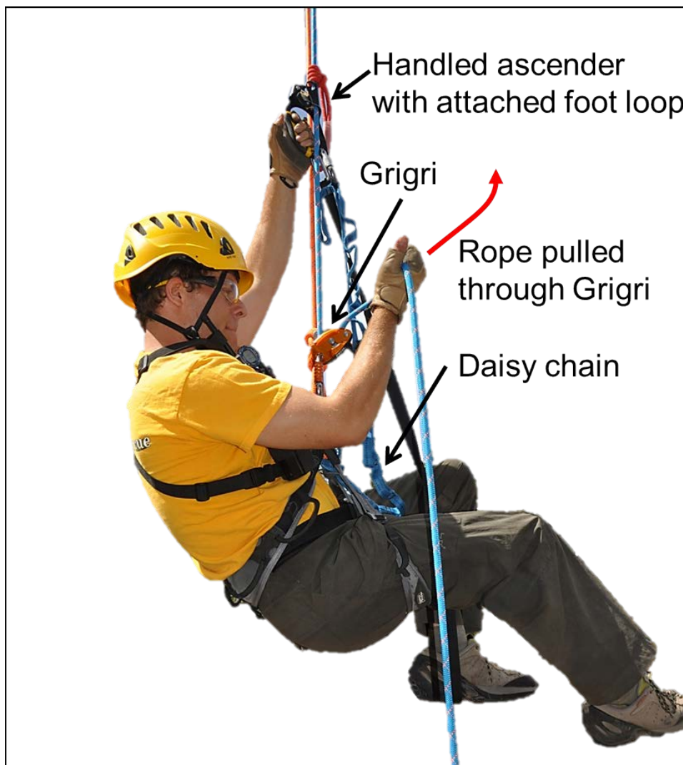
Figure 153- Grigri Ascending Technique
