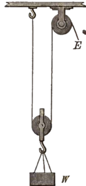
Figure 168- Mechanical advantage pulley system with fixed and moveable pulley. From First Principles of Physics . H. Carhart and H. Chute. 1912.
