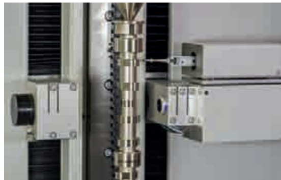
Tactile measuring unit with y-measuring axis 60 mm
