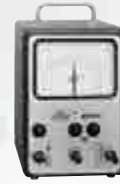
Millitron - Built in 1964. It is a compact length measuring instrument that was given the nickname "The Miner's Lamp"
