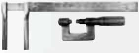
Vernier Calipers from Carl Mahr - Made of steel and brass, produced in 1868
