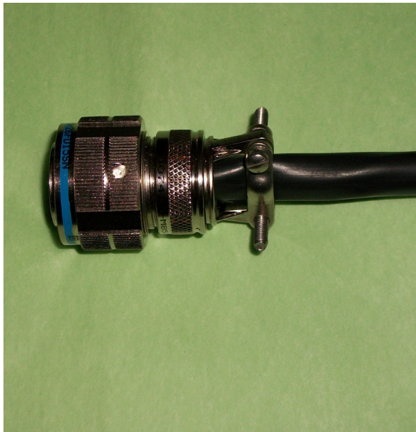
LOW VOLTAGE CABLE WITH MATING D38999/26FD15SN CABLE CONNECTOR
