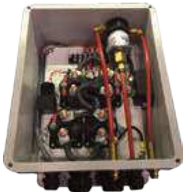
Hose Reel with Air Solenoid Control Unit Inside view
