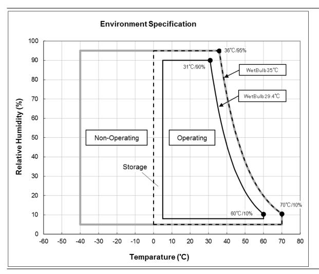
Figure 5 Limits of temperature and humidity
