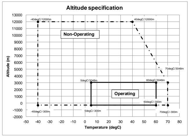
Figure 4 Limits of temperature and altitude
