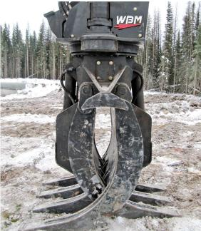
The WBM Clam (Powerclam) Grapple is a very versatile tool. With many options to choose from, this grapple can be configured to handle tree length, cut-to-length, shortwood, as well as brush piling and blow down with the cut-off saw arrangement. Bucket configurations are also available for road building and other bulk material handling applications.
