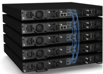
Figure 1: Brocade ICX 6610 Switches can be stacked using four standard 40 Gbps QSFP ports that provide a fully redundant virtual chassis backplane with 320 Gbps of stacking bandwidth.
