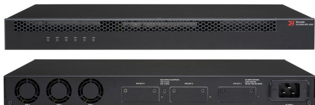
Figure 3: The optional Brocade ICX 6400-EPS1500 is an external power supply source to provide additional power to the Brocade ICX switches (except the Brocade ICX 6430-C, 6450-C, and 6430-24). It also can be used for system power redundancy and increased PoE/PoE+ power budget to enable additional PoE/PoE+ ports. Each Brocade ICX 6400-EPS1500 can connect up to three Brocade ICX 6430 and 6450 Switches.
