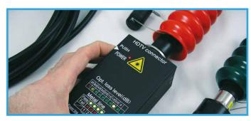
This cable tester provides a quick and easy means of checking the functionality of HD hybrid fibre cables and cable systems. A laser source checks the fibres giving an indication of the attenuation through the whole cable or cable system, and electrical tests check for continuity of both the power and control conductors.
