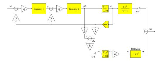
Figure 5.12: MASH structure with reduced sample-rate requirement for the second stage
