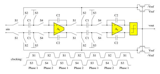
Figure 2.18: Switched-capacitor second-order delta-sigma ADC
