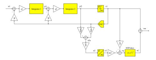
Figure 3.5: General structure of the cascaded 2-0 delta-sigma ADC
