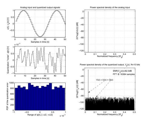
Figure 2.5: The spectrum of a quantized sinewave for N=10 bits
