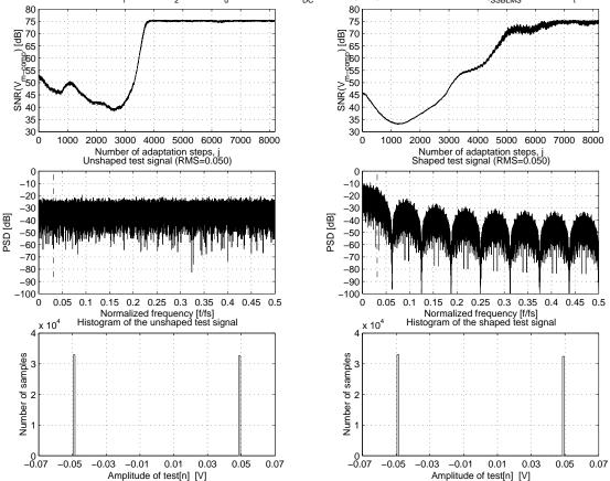
$\text{SSBLMS} @ \text{OSR=16}, \text{N}_1 = 1.5 \text{ bits}, \text{N}_2 = 10 \text{ bits}, \text{A}_u = 0.1 \text{V}, \Delta = 0.8 \text{W}, \text{A}_{\text{DC}} = 54 \text{dB}, \text{N}(\text{kT/C}) = -92 \text{dB}, \text{M} = 6, \text{K} = 65536, \text{Y}_{\text{SSBLMS}} = 1.5 \text{e} - 05, \text{A}_t = 0.05 \text{V}, \text{M} = 0.05 \text$
