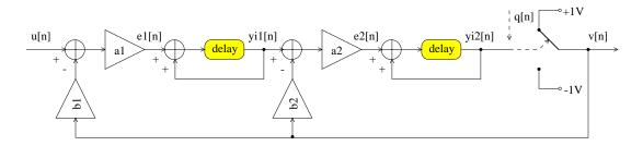
Figure 2.19: Time-domain model of the second-order delta-sigma ADC
