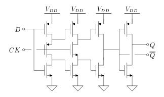
Figure 5.8: TSPC flip-flop used in the comparator
