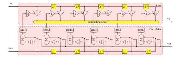
Figure 4.3: Simplified hardware implementation of the correlator using a binary test signal test[n] to update the coefficients  $l_i$  of the adaptive noise-leakage compensation digital filter  $L_C(z)$   $(q = \gamma_{SSBLMS} \text{ and } M - 1 = 5)$
