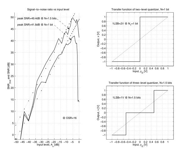
Figure 2.25: Comparative performance of bi- and tri-level modulators
