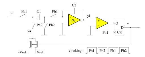
Figure 2.11: Switched-capacitor first-order delta-sigma ADC
