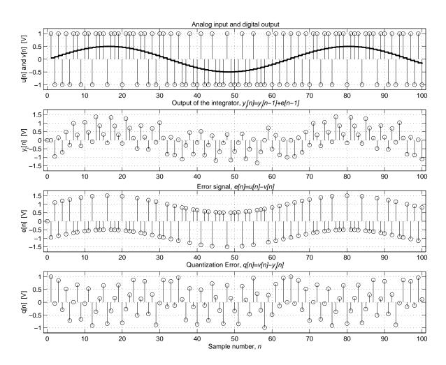
Figure 2.13: First-order delta-sigma ADC response in time to a half-scale in-band sinewave input (OSR = 32)
