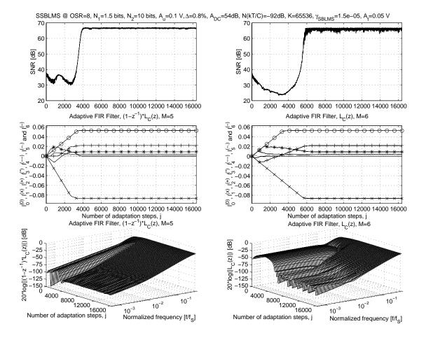
Figure 4.9: (a) Reducing the ripple of the adaptation noise using a differentiator, M = 6; (b) adaptation process without differentiator, M = 7
