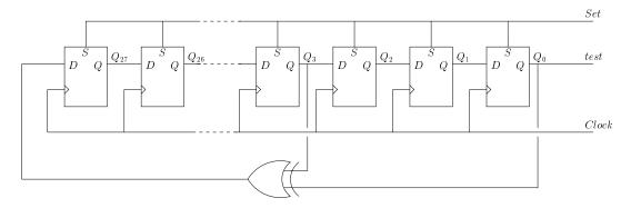
Figure 5.14: 28-bit maximum-length sequence generator
