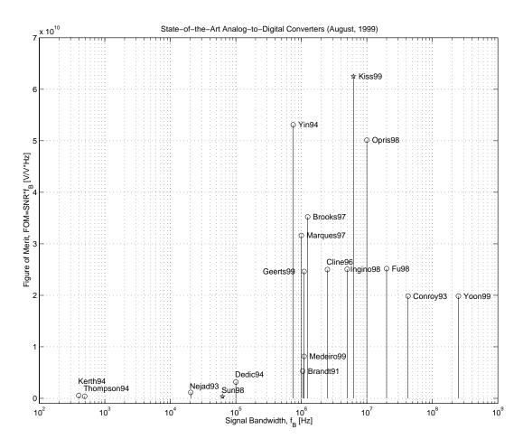
Figure 1.2: Figure of merit for state-of-the-art ADCs
