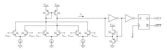
Figure 5.7: Comparator used in the tri-level quantizer
