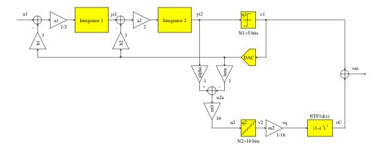
Figure 4.13: High-performance 2-0 MASH ADC
