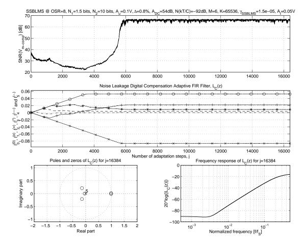
Figure 4.5: Adaptive compensation process ( $K = 2^{16}, \gamma_{SSBLMS} = 1.5 \, 10^{-5}$ )
