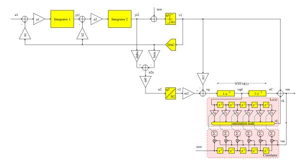
Figure 4.8: Improved adaptive digital noise-leakage compensation scheme using a test signal test[n] for the general cascaded 2-0 delta-sigma ADC
