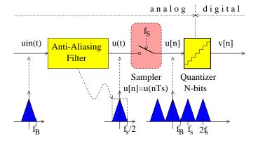
Figure 2.1: General analog-to-digital converter
