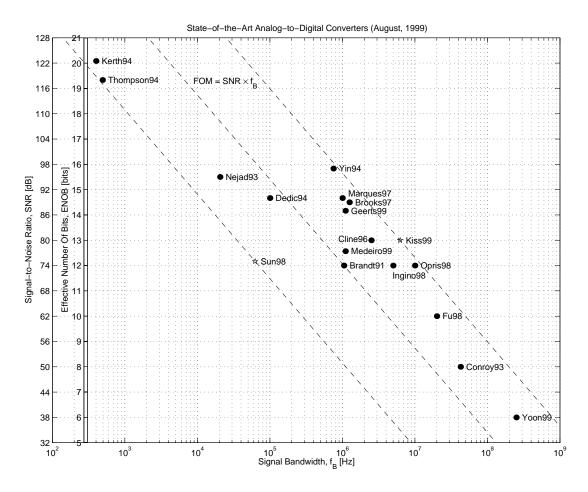
Figure 1.1: State-of-the-art ADCs (August, 1999)
