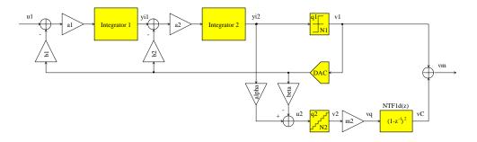
Figure 3.2: Standard structure of the cascaded 2-0 delta-sigma ADC
