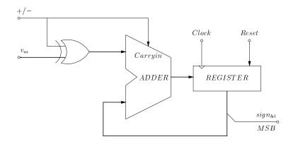
Figure 5.13: Accumulator for the adaptive filter
