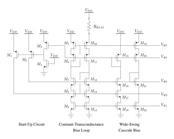
Figure 5.5: Generation of the bias voltages for the opamps
