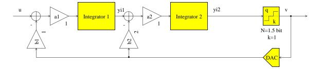
Figure 2.24: Second-order tri-level delta-sigma ADC
