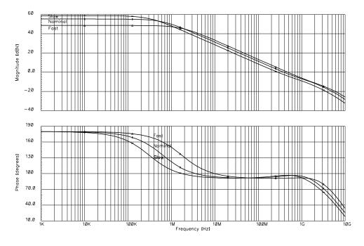
Figure 5.15: Operational amplifier frequency response
