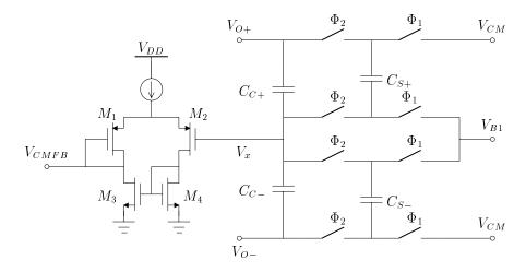
Figure 5.4: Common-mode feedback circuit for the opamps
