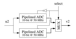
Figure 5.11: Time-interleaved 2 pipelined ADC implementing the second-stage quantizer
