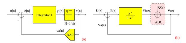
Figure 2.10: (a) First-order delta-sigma ADC and (b) its linearized model
