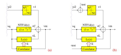
Figure 4.1: Adaptive digital noise-leakage compensation (a) without and (b) with a test signal test[n]
