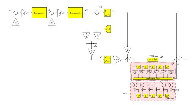
Figure 4.2: Adaptive digital noise-leakage compensation scheme using a test signal test[n] for the general cascaded 2-0 delta-sigma ADC (M = 6)
