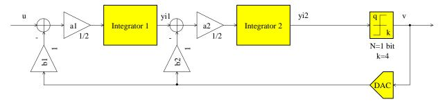
Figure 2.14: Second-order single-bit delta-sigma ADC
