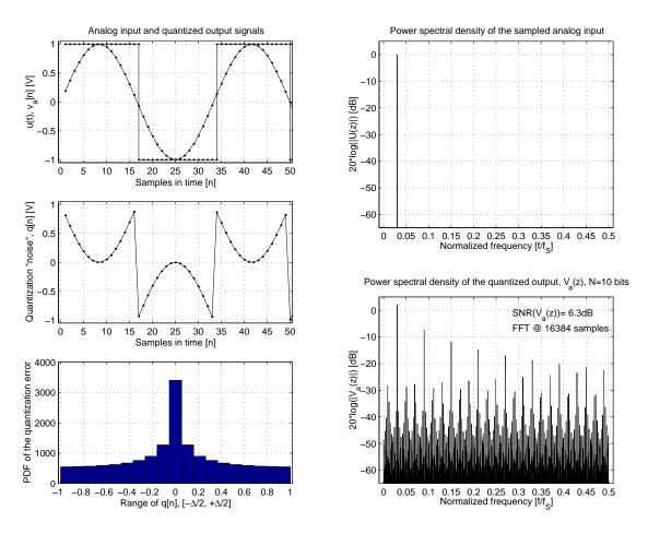
Figure 2.9: The spectrum of a quantized sinewave for N=1 bit
