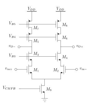
Figure 5.3: Telescopic opamp schematic used in the integrators
