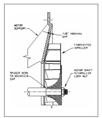
Figure 6-1 Impeller Cutaway
