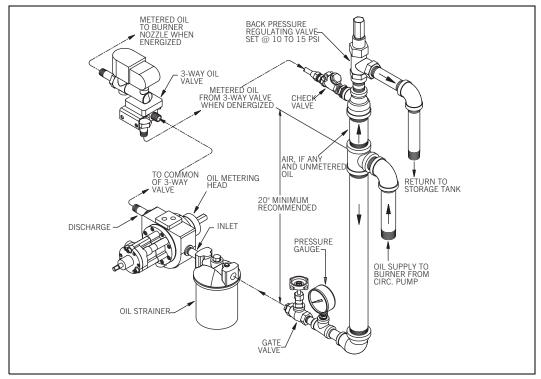
Figure 5-18 Typical Oil Supply Loop
