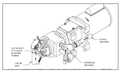
Figure 5-16 Separate Fuel Oil Metering Pump
