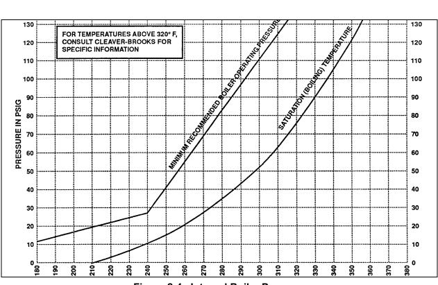
Figure 2-4. Internal Boiler Pressure
