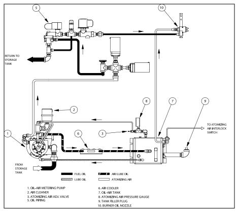
Figure 5-13 Integral Compressor Oil-Air Metering System
