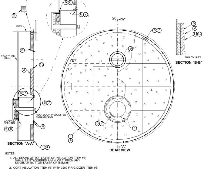
COAT INSULATION (ITEM #5) WITH 3200 F RIGIDIZER (ITEM #3) MIXED WITH WATER TO A 50:50 SOLUTION, APPROXIMATELY 1/4" DEEP, AFTER SCREEN IS INSTALLED.
