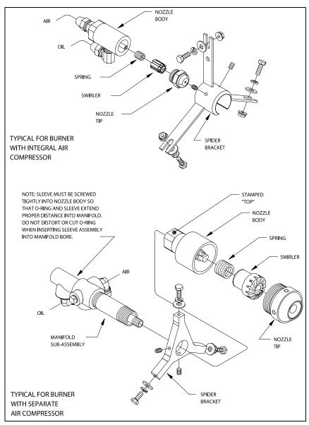
Figure 6-4 Oil Nozzle Assemblies
