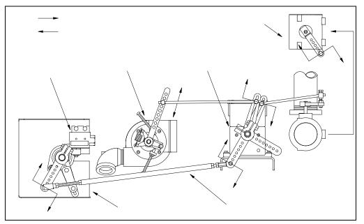
Figure 6-6 Firing Rate Controls
