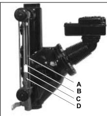
A. Normal level of water: feed pump turns off at this point. Fill pressure vessel initially to this height.
