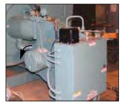
Figure 4-1 Motor and Fan Rotation
