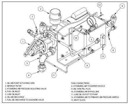
Figure 6-7 Integral Oil Air Metering System and Tank
