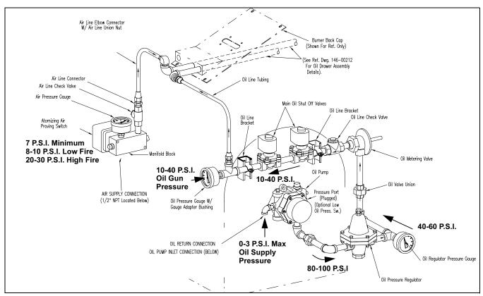
Figure 4-9 Light Oil Piping, Direct Drive
