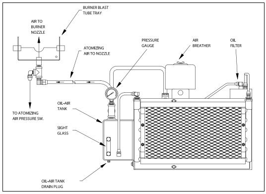
Figure 5-19 Separate Compressor Module
