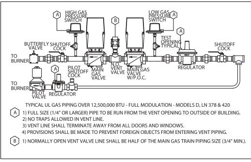
Figure 5-20 Typical UL Gas Train Over 12.5 MMBtu, Full Modulation
