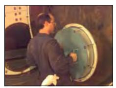
Figure 2-13 Removing Rear Access Plug
