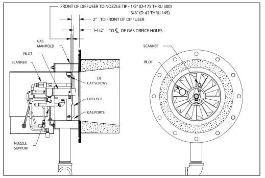
Figure 6-5 Firing Head Assembly
