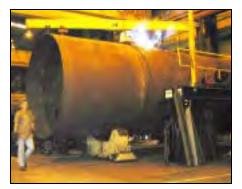
Figure 1-8 ASME Welding on a Firetube Pressure Vessel
