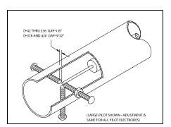
Figure 6-2 Gas Pilot Electrode
