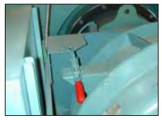
Figure 5-10 Housing Swing Latch
