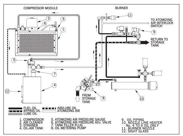
Figure 5-17 Separate Compressor - Air Metering System
