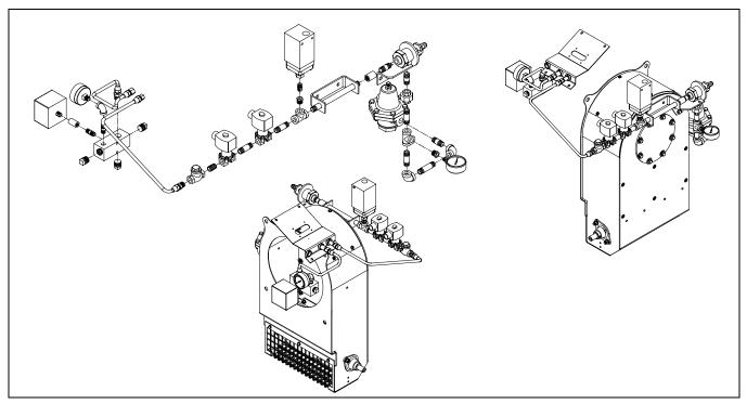
Figure 4-10 Typical Arrangement for Remote Oil Pump with Air Atomization
