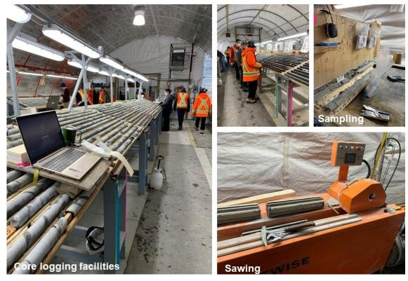
Figure 12.2 – Core logging facilities and sawing room at the Fenelon Camp
