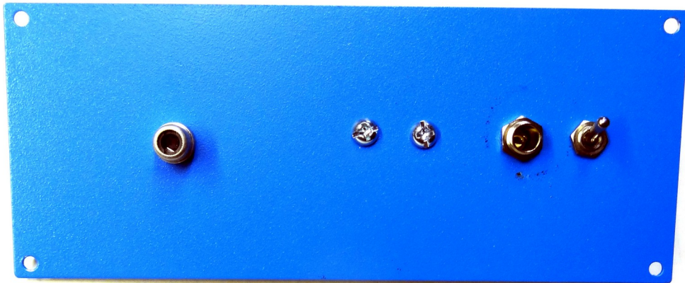
The rear panel showing the RCA output connector, the coaxial power input, and the power switch.
