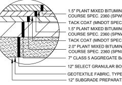
1.5" PLANT MIXED BITUMINOUS WEARING COURSE SPEC. 2360 (SPWEA240C) TACK COAT (MNDOT SPEC. 2357) 1.5" PLANT MIXED BITUMINOUS WEARING COURSE SPEC. 2360 (SPNWB240C) TACK COAT (MNDOT SPEC. 2357) 2.0" PLANT MIXED BITUMINOUS NON-WEARING COURSE SPEC. 2360 (SPNWB230B) 7" CLASS 5 AGGREGATE BASE, SPEC. 2211 12" SELECT GRANULAR BORROW, SUBBASE SPEC. 3149.2B1 GEOTEXTILE FABRIC, TYPE 5 (NON-WOVEN), SPEC. 3733 - 12" SUBGRADE PREPARATION-MNDOT 2112 (INC.)
