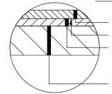
1.5" PLANT MIXED BITUMINOUS WEARING COURSE SPEC. 2360 (SPWEA240C) TACK COAT (MNDOT SPEC. 2357) 1.5" PLANT MIXED BITUMINOUS WEARING COURSE SPEC. 2360 (SPNWB240C)
