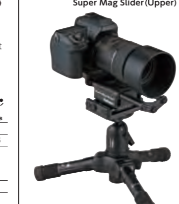
Super Mag Slider For macro photography, for finely adjusting the frame forward and back, left and right. Upper unit for forward and back can be detached to use separately. L: 210(8.27) x W: 120(4.72) x H: 70(2.76) mm(inch) Maximum adjustment: Forward/back: 60mm/2.36inch Left/right: 30mm/1.18inch Weight: 470g/1.04lbs UNC 1/4 & 3/8 tripod socket JAN/EAN 4907990 273253 UPC 017915 884052
