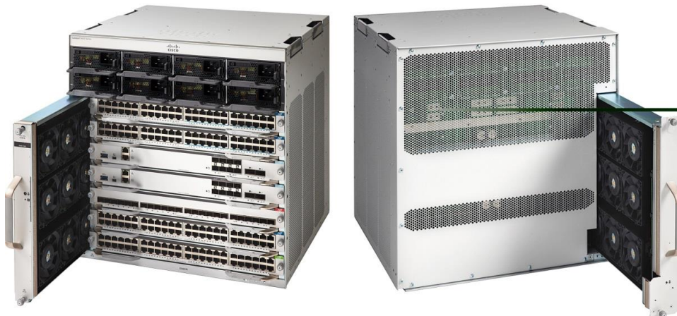
Figure 2. Dual serviceable fan tray
