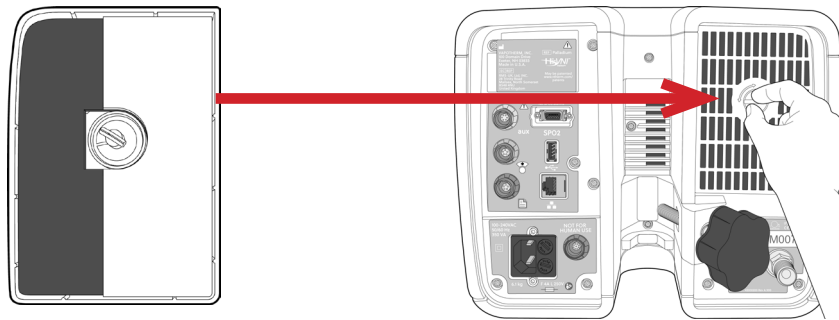
Figure 53: Insert patient air intake filter in back of device
