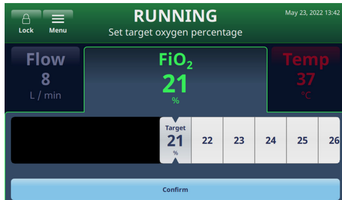
Figure 29: Setting FiO 2 parameter using the scroll bar
