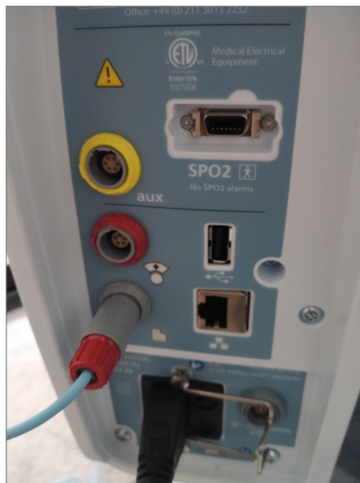
Figure B1: HVT 2.0 EMR Link Cable placed in EMR data port
