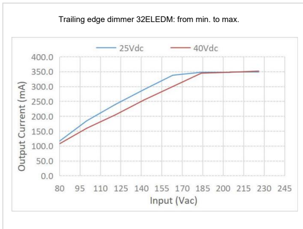
Triac Dimming Curve 3
